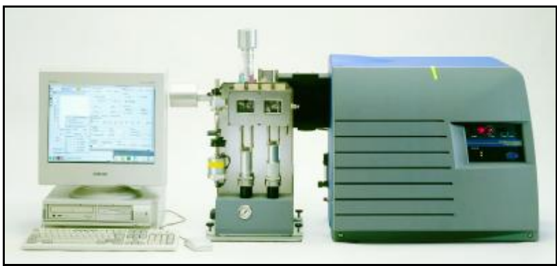
PiStar-180 configured for stopped-flow kinetic measurements
