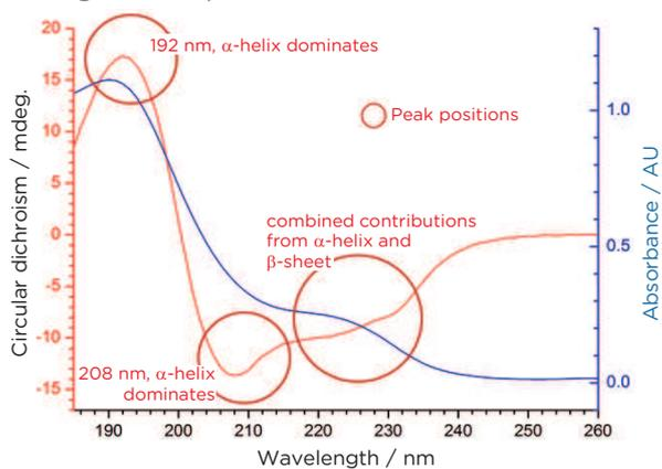
Simultaneous acquisition of CD and absorbance spectra, 0.5 mm pathlength, Chirascan V100. Courtesy of leading research university, Germany
