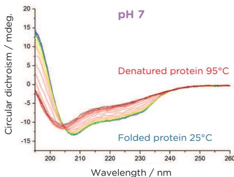
Two of six denaturation datasets acquired at pH 2-7, lysozyme, Chirascan 6-cell turret, Chirascan V100, raw data, no baseline adjustment, no smoothing, 0.5 mm pathlength
