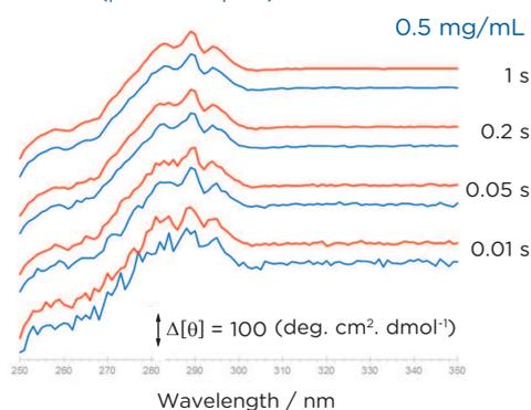
Tertiary structure of lysozyme – raw data, no smoothing, baseline corrected, n=3 scans, 1 nm step, 10 mm pathlength, spectra offset for clarity
