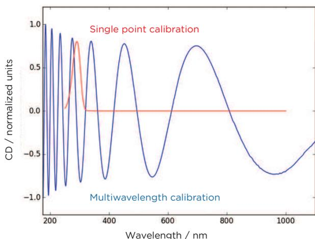
Conventional chemical calibration methods require considerable skill in preparation. Standards, such as camphor-10-sulfonic acid (CSA), are unstable, photolabile and hygroscopic. In addition, single wavelength calibration (290.5 nm) assumes the same linear response at all wavelengths.
