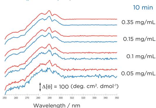
Tertiary structure of lysozyme – raw data, no smoothing, 10 min. baseline / 10 min. sampling, n=3 scans, 0.5 nm step, 10 mm pathlength, spectra offset for clarity
