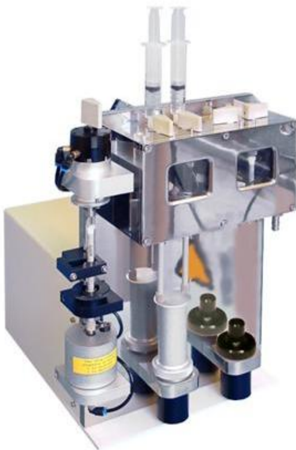
Figure 2-7: sequential-mixing SHU in single-mixing configuration
