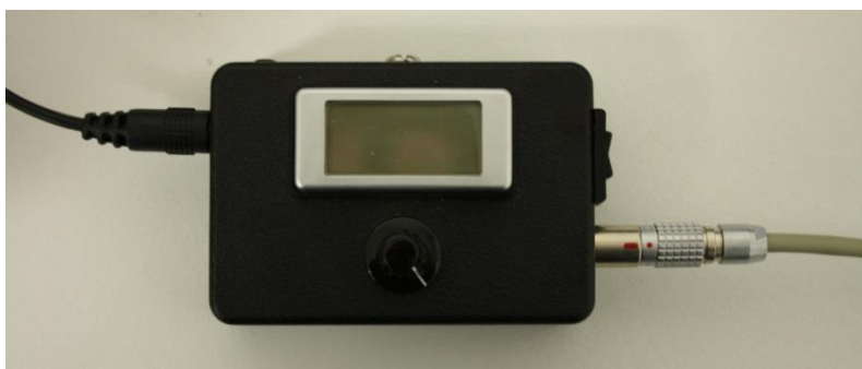
Figure 3-18: The LED Power Supply
