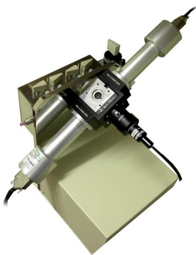
Figure 2-21: the fluorescence polarisation accessory (Note: This image is for an SX20 system equipped with a monochromator. The unit for an SX20-LED system will look slightly different to this)
