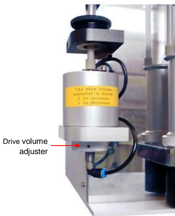
Figure 2-9: the location of the drive column adjuster on the stop mechanism
