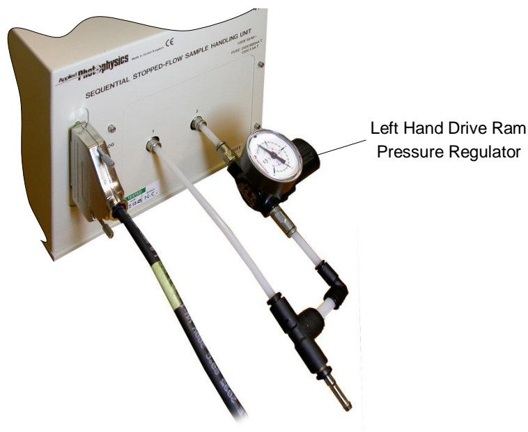
Figure 3-37: position of the drive pressure regulator on the rear of the SHU
