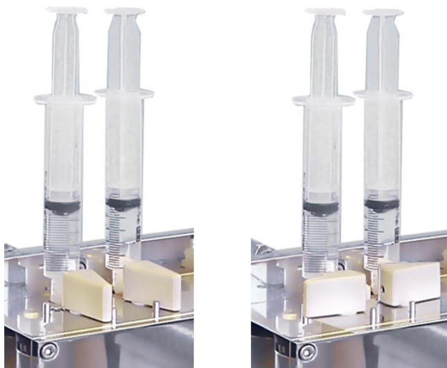
Figure 3-9: drive valves in Drive position (left) and Load position (right)
