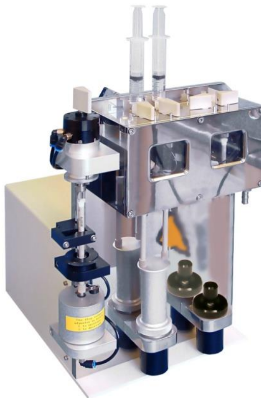
Figure 3-31: sequential-mixing SHU in single-mixing configuration
