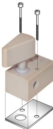
Figure 3-8: a right hand drive valve
