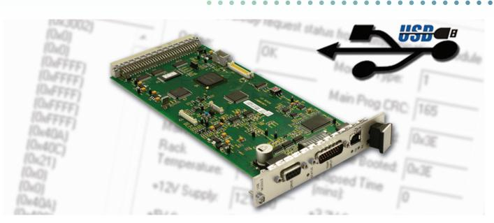
The USB communications upgrade is a requirement for operation of Applied Photophysics instruments with Windows 7, 8 and 10. It replaces older fibre-optic communications on instruments supplied between 2004 and 2010 operating under Windows XP.
