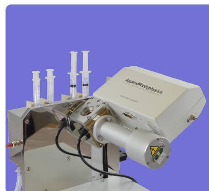
LED Light Source fitted to the instrument
