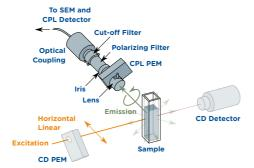
CD PEM: inactive, produces horizontall linear polarized light
