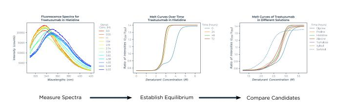
The SUPR-CM offers a simple to use solution for running chemical denaturation experiments. Compatible with both 96 and 384-well microplates, the SUPR-CM is a flexible platform. Run chemical denaturation experiments with more denaturant concentrations to improve measurement resolution. Being both plate-based and leveraging intrinsic fluorescence, the SUPR-CM has low sample requirements without compromise on measurement performance.
