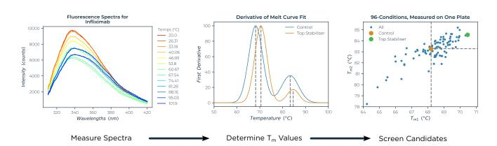
The SUPR-DSF can leverage the natively high capacity of the 384-well PCR microplate to screen hundreds of samples/conditions at a time. Coupled with commercially available screening plates. The SUPR-DSF helps reduce the workload of sample preparation, maueasurement and processing of the thermal denaturation curves. All while working at low sample requirements and with less consumable costs.
