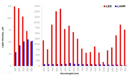
The intensity of each LED compared to an equivalent wavelength and bandwidth output from the standard xenon light source is shown in the figure above. The higher intensity LEDs used as an excitation source for fluorescence measurements produce a considerable increase in emission intensity. As a consequence, detection sensitivity and signal-to-noise levels are improved.
