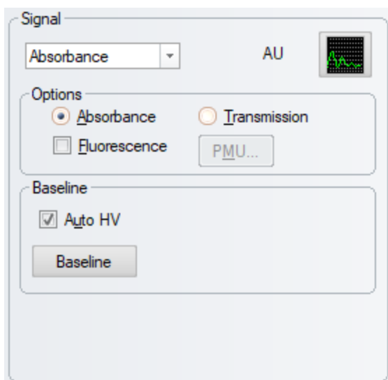
Figure 34: The Signal panel with Absorbance selected
