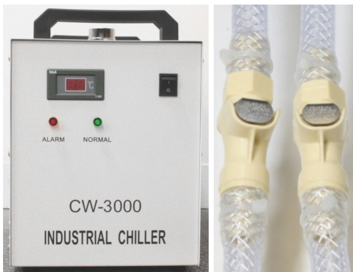
Figure 19: The water circulator (left) and circulator quick release fittings (right)
