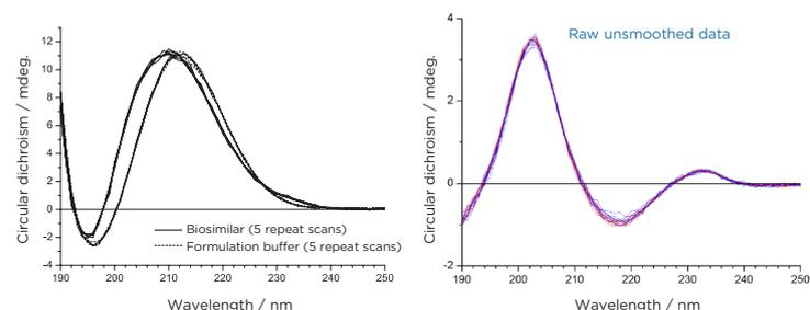
Risk of baseline artefacts removed by dialysis of biosimilar and innovator lots against a common preparation of formulation buffer and using formulation buffer as reference.
